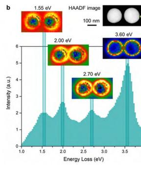
A scanning transmission electron microscope (STEM) can probe localized surface plasmons with nanometer spatial resolution and ultra-high energy resolution using electron energy loss spectroscopy (EELS).
