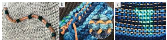
Figure 6: Demonstration of three textile integration techniques with electronic yarn. (a) Hand-embroidery. (b) Hand-knitting. (c) Weaving.
