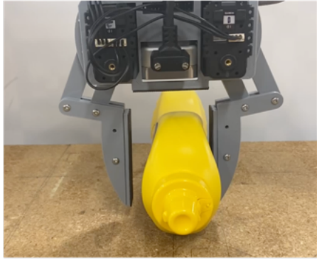
Fig. 4. Gripper grasping the mustard container from the YCB dataset from an off-center position (left). Limiting torque during approach prevents the mustard from moving as the right finger makes contact. Dashed vertical lines indicate contact by the right finger, contact with both fingers, and opening (from left to right).
