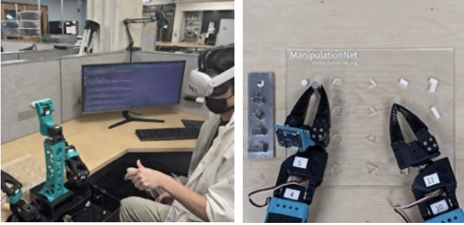
Fig. 9. VR Teleoperation Setup: (Left) The operator interacting with the system; (Right) a detailed view of the ManipulationNet peg-in-hole board.
