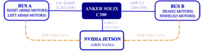
(a) Logical power schematic
